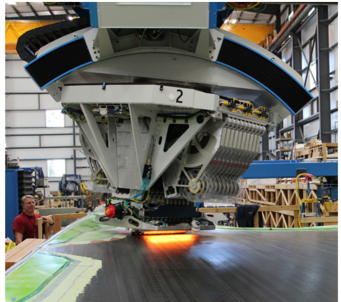
Figure 1. 20 Tow, 1.5 Inch AFP Head Depositing Carbon on Prototype Wing Tool during Development.
